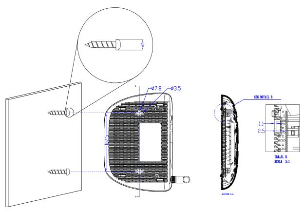
Figure 2-1 Wall-mount Install
